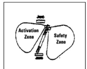
In case of power failure, the Magic-Force™, Magic-Access™ and Magic-Swing™ operators function as manual door closers in the direction of swing. Magic-Force™ and Magic-Access™ are also available with a light-duty spring for applications that require a lower force for manual exit.
