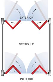
Our door panels fold in or out for the most efficient use of space at entrances or exits.
